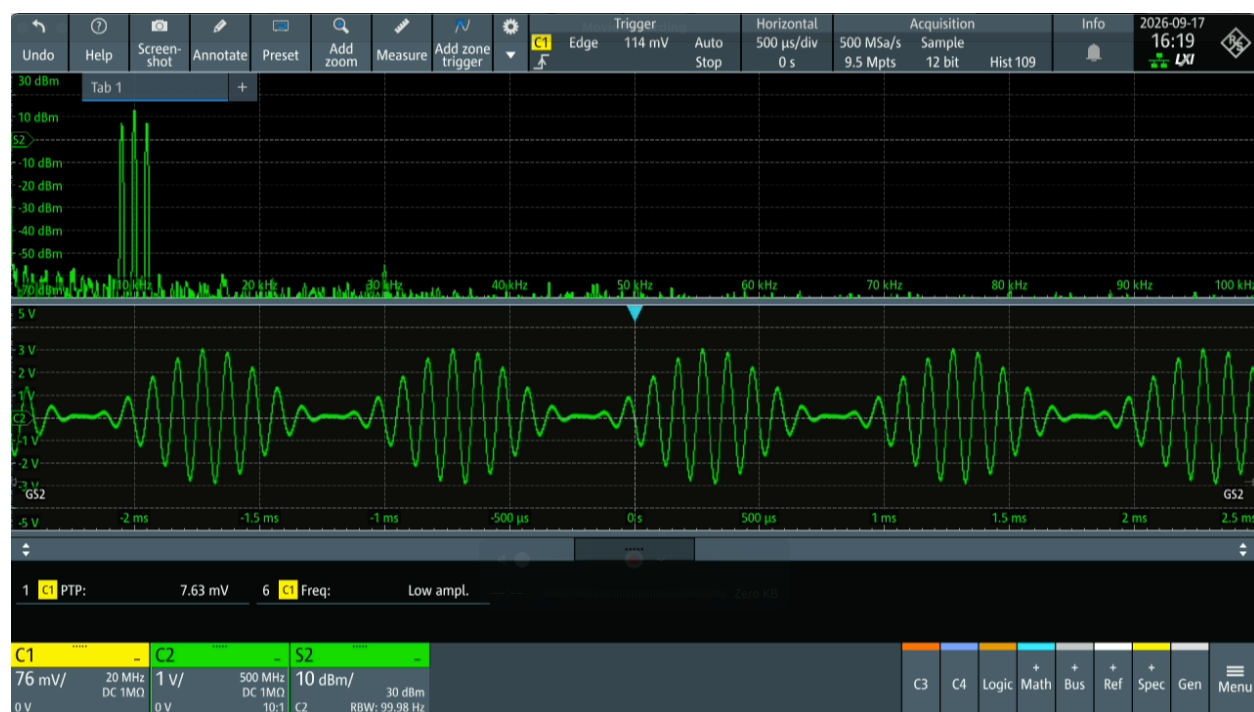
Figure 13: Example of 10kHz carrier, 1kHz AM frequency and 100% modulation depth using the code in Appendix 3. The top trace is the AM spectrum, the bottom is the time-domain signal. Note that no visible spurs appear out to 100kHz.
