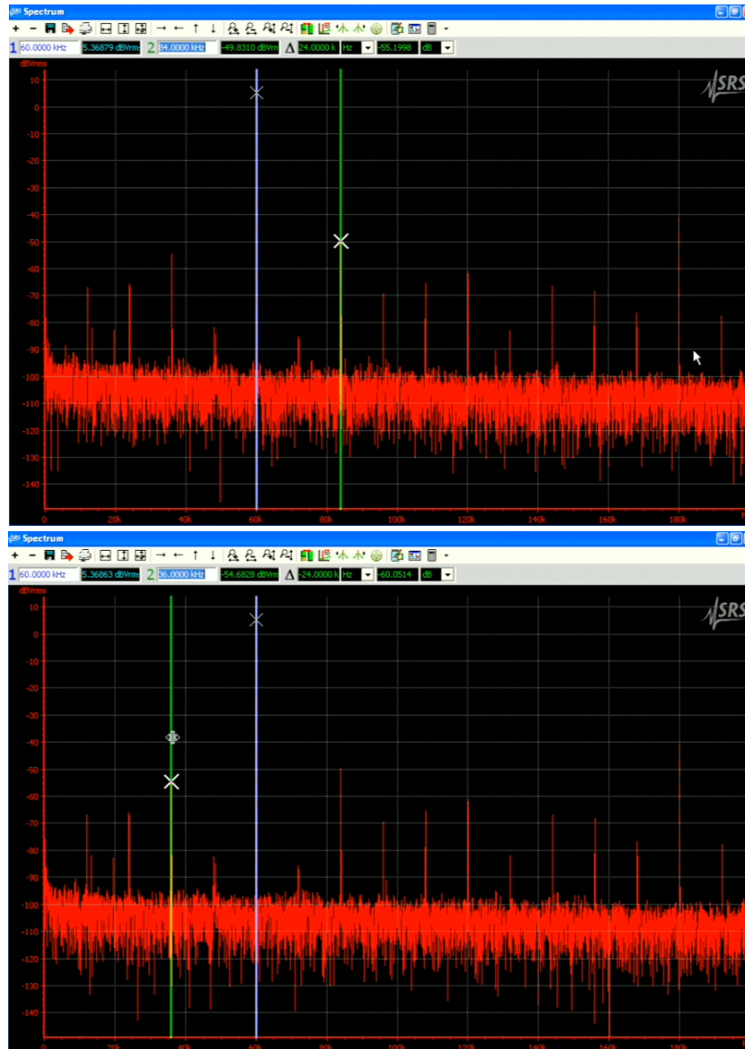
Figure 9: High-frequency view of 60 kHz output and accompanying spurs, with the SR1 in high-frequency mode, showing frequencies up to 128 kHz. Note many spurs above the band of interest (top image) and in-band (lower image). At this point the PCM5102A is way out of its designed-for frequency range of operation, but still doing a great job!
