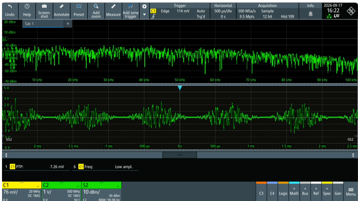
Figure 15: Example of 100% AM modulated random noise, with the same modulation parameters as in Figure 13.
