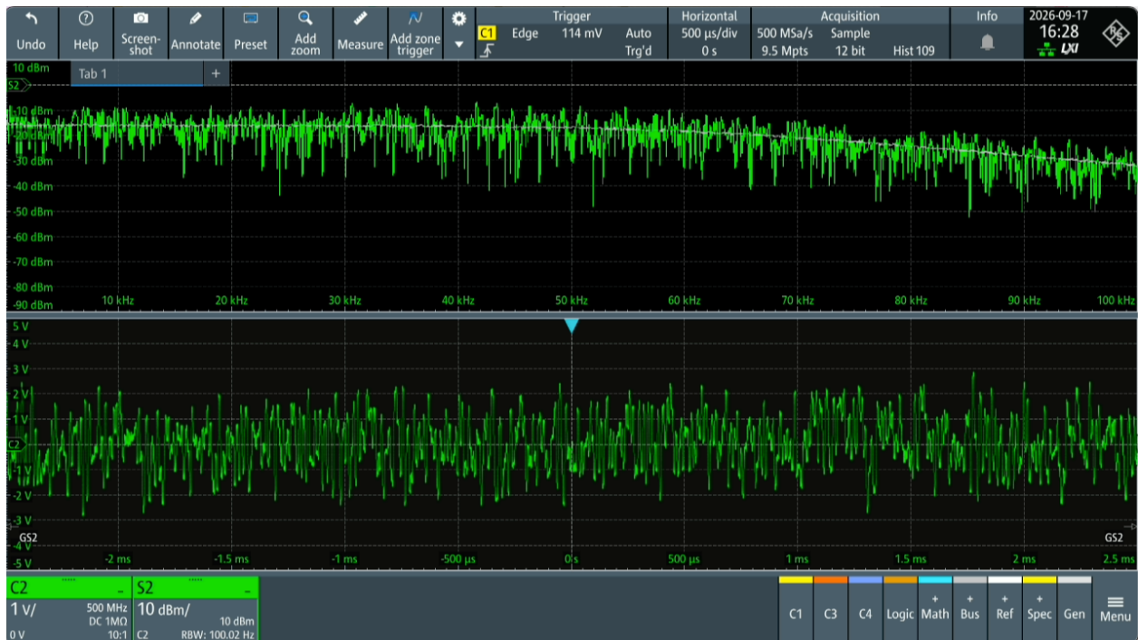
Figure 14: Random noise output, unmodulated (bandwidth is shaped by the output filter). The white trace is the average of the spectrum, which is very flat out to the target 60kHz bandwidth (detailed measurements showed that the noise is down 1dB by 50 kHz).
